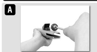
Tighten head mounting screw with a screwdriver(No.2) sold separately.
