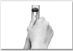
Bend the arm to the right or left and adjust, so that the head touches the center line of the main body.
